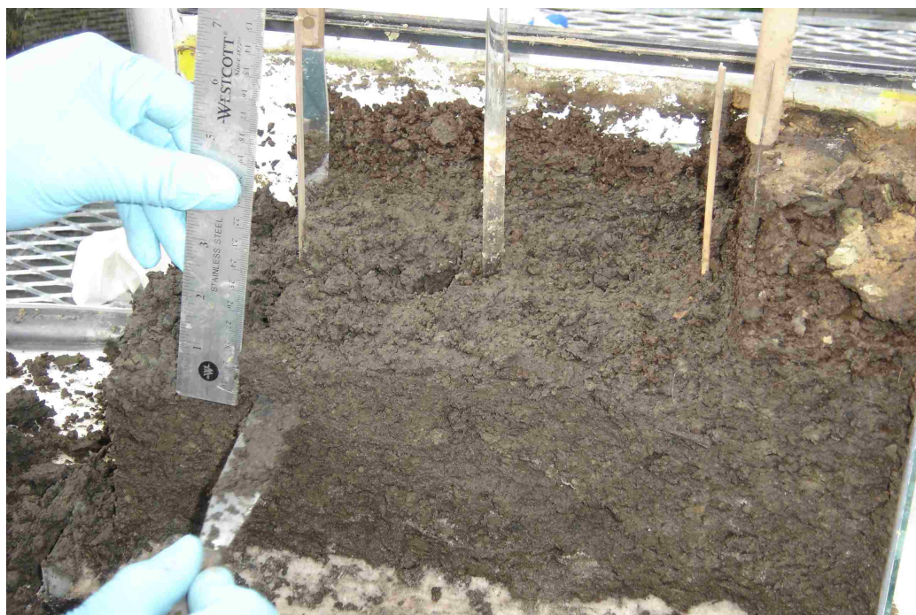
Figure 3.5. An example of the reactor sampling. The measurement of each soil layer is done using a ruler before removal using sterilized spatulas. The dowels mark the location of the soil cores taken throughout the experiment.
